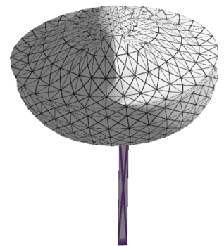
Figure 25: The balloon inflates from a bowl shape to a spherical shape.
